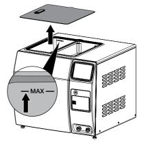
Fill the fresh water container with distilled or demineralised water to the MAX mark (approx. 4 litres).
