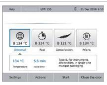
The sterilisation chamber is automatically preheated to 121 °C in the default settings.
