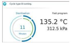
Saturated steam is generated inside the steriliser chamber until the specified values are reached. The actual sterilisation takes place during the predefined hold time. At the end of the sterilisation phase the steam is let off.
