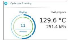
The parts for sterilisation in the sterilisation chamber are dried under vacuum. Afterwards the sterilisation chamber is vented via the sterile air filter and the door can be opened.
