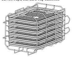
The carrier can be loaded with up to 6 trays or - rotated through 90° - 3 standard tray cassettes.
